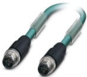
Assembled Ethernet cable, CAT5e, shielded, 2-pair, 26 AWG stranded (7-wire), RAL 5021 (water blue), M12 plug to M12 plug, line, length 3 m
