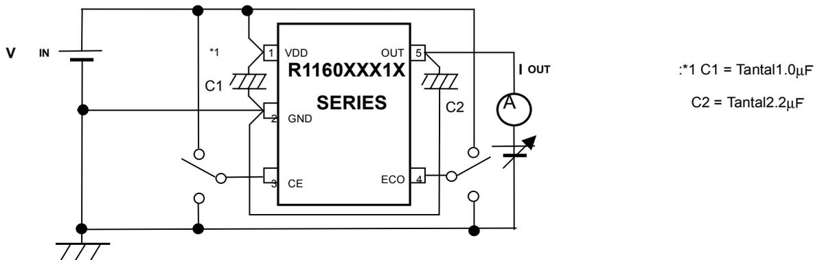
Fig.1 Output Voltage vs. Output Current Test Circuit
