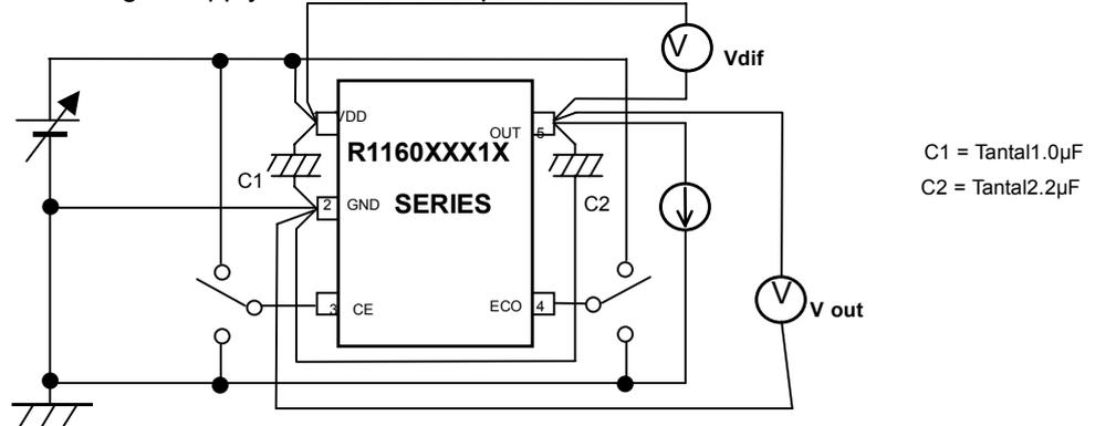
Fig. 6 Dropout Voltage vs. Output Current/ Set Output Voltage Test Circuit
