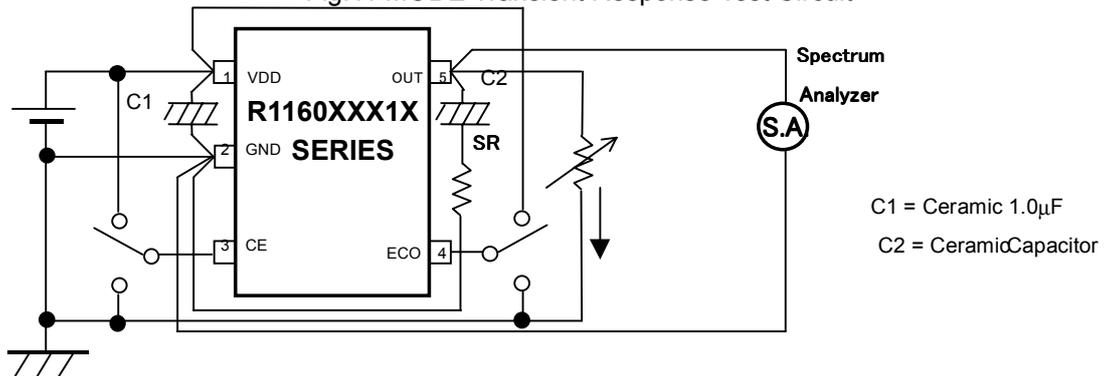
Fig.12 Output Noise Test Circuit(IOUT vs. ESR)
