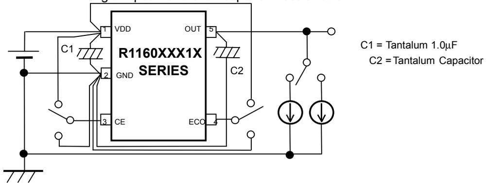
Fig.9 Load Transient Response Test Circuit
