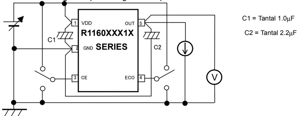
Fig.2 Output Voltage vs. Input Voltage Test Circuit
