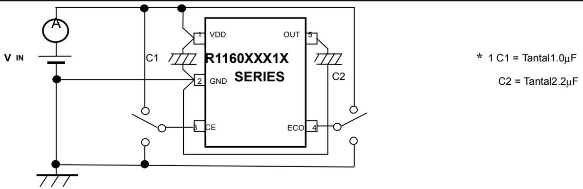
Fig.3 Supply Current vs. Input Voltage Test Circuit
