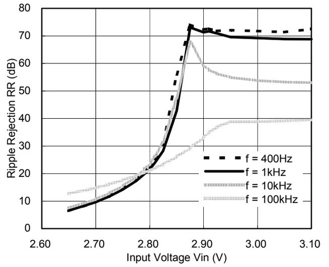
9) Ripple Rejection vs. Frequency
