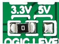
RF Meter click has an SMD jumper (zero ohm resistor) for setting the logic level either at 3.3V or 5V.
