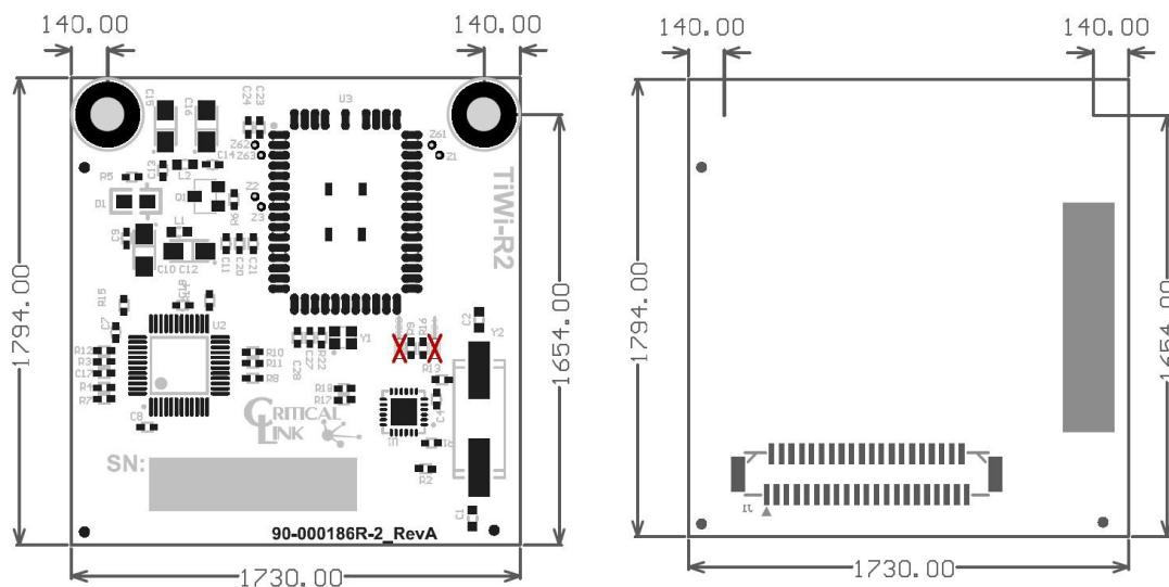
Figure 1: Dimensions 1.73" x 1.79" – Top and Bottom Mechanicals
