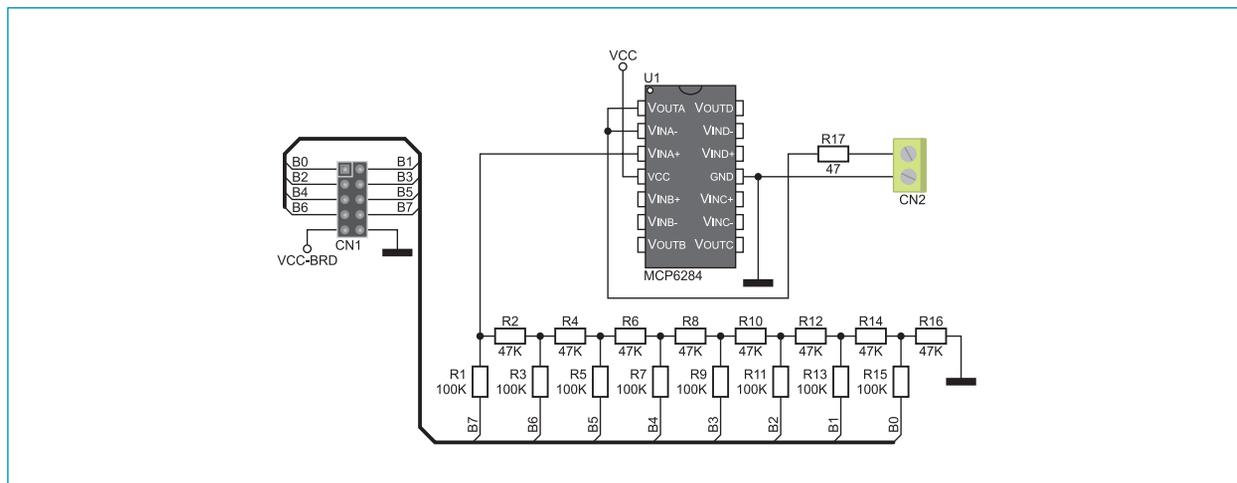
Figure 2: R2R DAC additional board connection schematic
