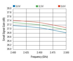
Figure 5. Small Signal Gain vs Frequency across Vcc
