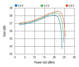
Figure 6. Gain vs Power Out Across Vcc
