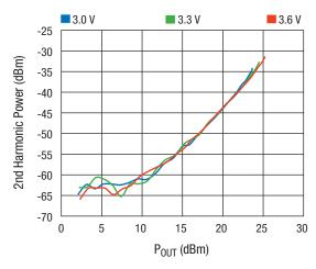
Figure 18. 2nd Harmonic vs. Power Out Across Vcc
