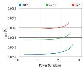
Figure 28. IREF vs Power Out Across Temperature
