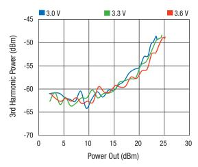
Figure 20. 3rd Harmonic vs. Power Out Across Vcc
