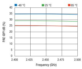
Figure 12. PAE @ P1dB vs Frequency Across Temperature
