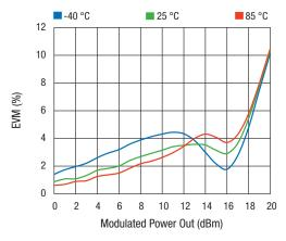
Figure 33. EVM vs Modulated Power Out Across Temperature 802.11g, 54 Mbps, 64 QAM
