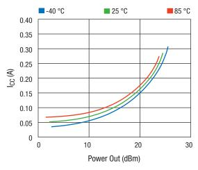
Figure 27. Icc vs Power Out Across Temperature
