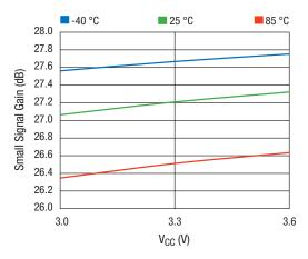
Figure 3. Small Signal Gain vs Vcc Across Temperature
