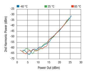
Figure 17. 2nd Harmonic vs. Power Out Across Temperature
