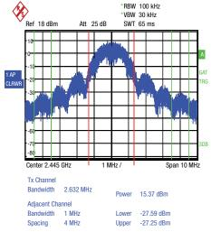
Channel Absolute Power Spectral Density at Mask Limit (absolute limit of -30 dBm with lf-fcl > 3.5 MHz with 100 MHz resolution bandwidth).
