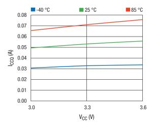
Figure 14. Iccq vs. Vcc Across Temperature
