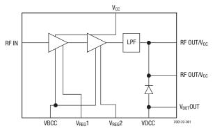
Figure 1. SKY65006-348LF Functional Block Diagram
