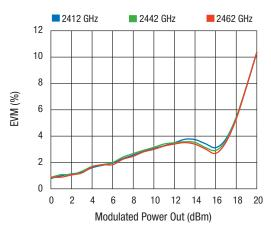
Figure 35. EVM vs Modulated Power Out Across Frequency 802.11g, 54 Mbps, 64 QAM
