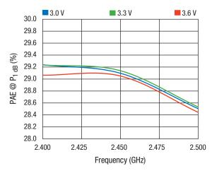
Figure 10. PAE @ P1dB vs Frequency Across VCC
