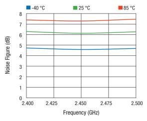
Figure 25. Noise Figure vs Frequency Across Temperature
