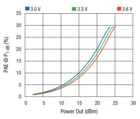
Figure 16. PAE @ P1dB vs Power Out Across Vcc
