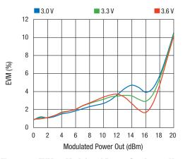
Figure 36. EVM vs Modulated Power Out Across Vcc 802.11g, 54 Mbps, 64 QAM
