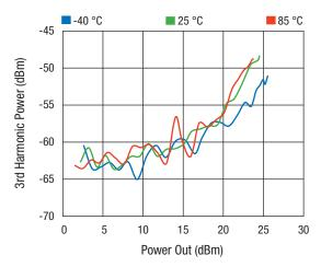
Figure 19. 3rd Harmonic vs. Power Out Across Temperature
