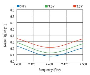
Figure 23. Noise Figure vs. Frequency Across Vcc
