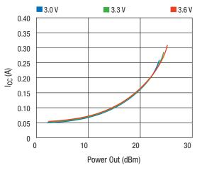
Figure 29. Icc vs Power Out Across Vcc
