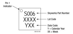
**Figure 43. Typical Package Marking**
