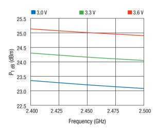
Figure 24. Output P1dB vs Frequency Across Vcc
