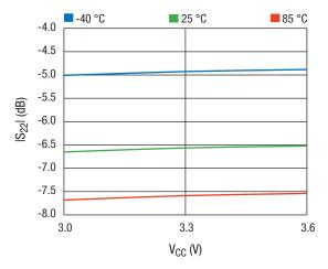
Figure 13. IS22I vs. Vcc Across Temperature
