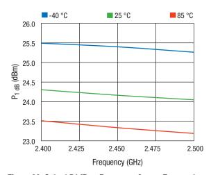
Figure 26. Output P1dB vs Frequency Across Temperature
