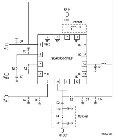
Figure 39. SKY65006-348LF Evaluation Board Application Schematic
