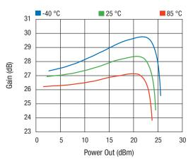
Figure 4. Gain vs Power Out Across Temperature
