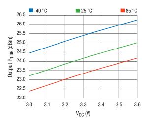
Figure 22. Output P1dB vs. Vcc Across Temperature
