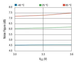
Figure 21. Noise Figure vs. Vcc Across Temperature
