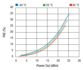
Figure 15. PAE @ P1dB vs Power Out Across Temperature
