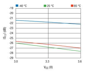
Figure 11. |S11| vs. VCC Across Temperature
