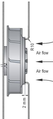
The air flow and noise level of fans without external housing depends on the installation conditions. The stated air flow and noise has been measured under the following conditions:
