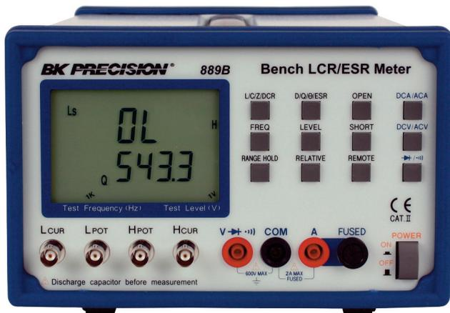
The B&K Precision 889B synthesized in-circuit bench LCR/ESR meter is a high accuracy test instrument used for measuring inductors, capacitors and resistors with a basic accuracy of 0.1%. Also, with the built-in functions of DC/AC Voltage/Current measurements and Diode/Audible Continuity checks, the 889B can not only help engineers and students to understand the characteristics of electronics components, but also being an essential tool on any service bench.
