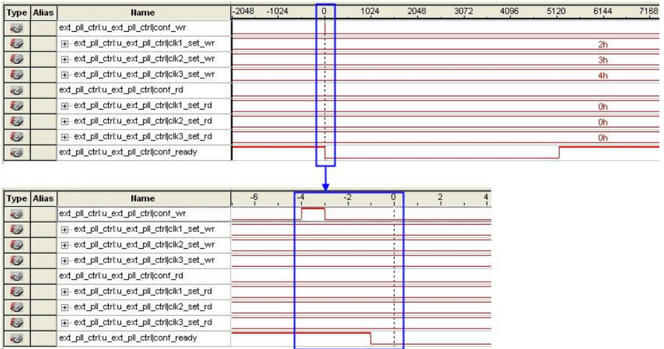
Figure 5-3 Write Timing Waveform
