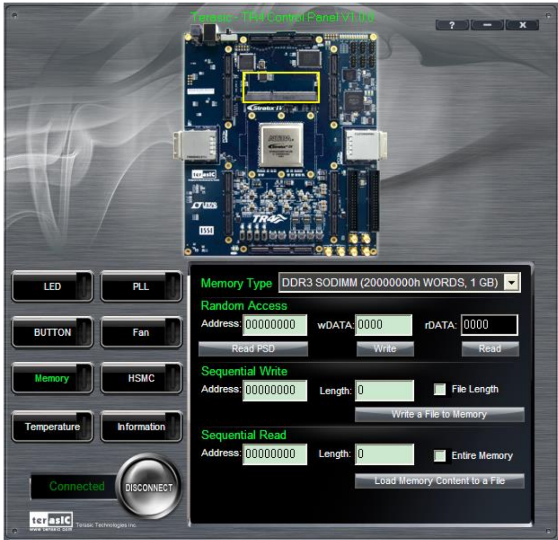
Figure 3-7 Access DDR3 SO-DIMM Memory
