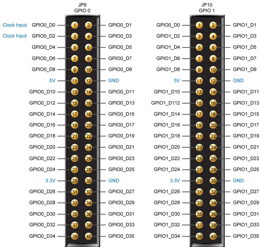
Figure 2-21 Pin Distribution of the GPIO Expansion Headers
