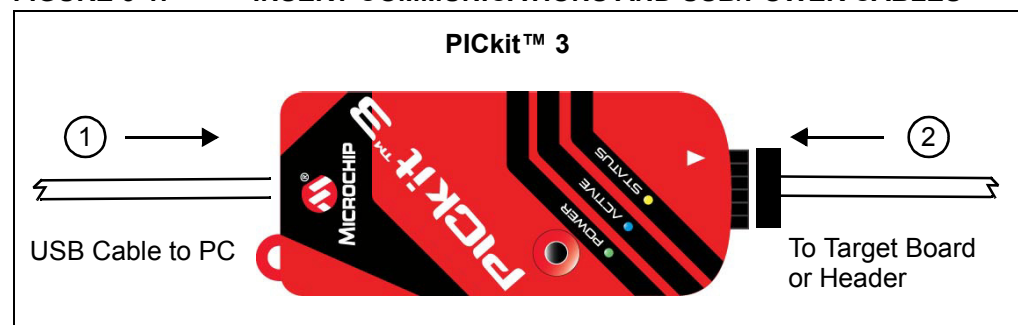
FIGURE 3-1: INSERT COMMUNICATIONS AND USB/POWER CABLES
