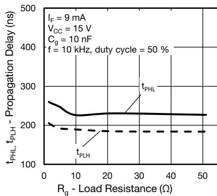
Fig. 20 - Propagation Delay vs. Load Resistance
