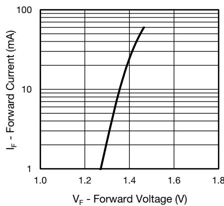
Fig. 6 - Forward Current vs. Forward Voltage
