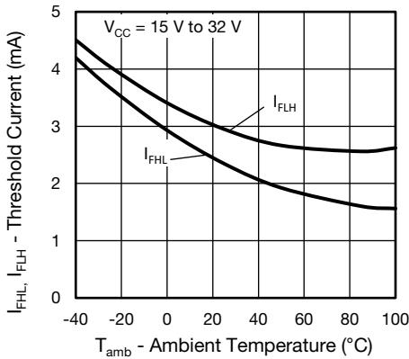
Fig. 15 - Threshold Current vs. Ambient Temperature
