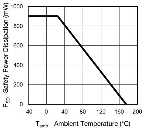
Fig. 1 - Safety Power Dissipation vs. Ambient Temperature
