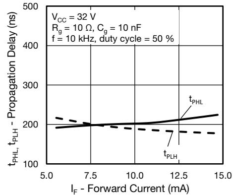
Fig. 19 - Propagation Delay vs. Forward Current
