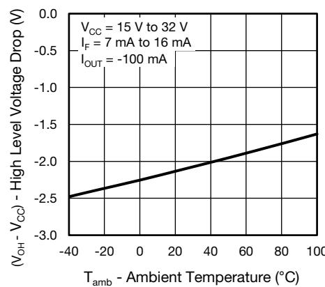
Fig. 7 - High Level Voltage Drop vs. Ambient Temperature
