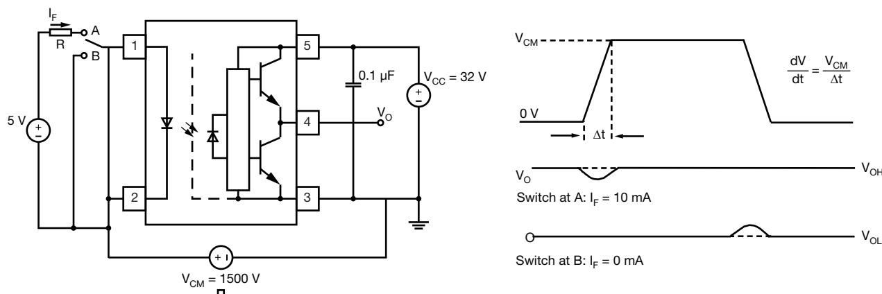
Fig. 5 - CMR Test Circuit and Waveforms
