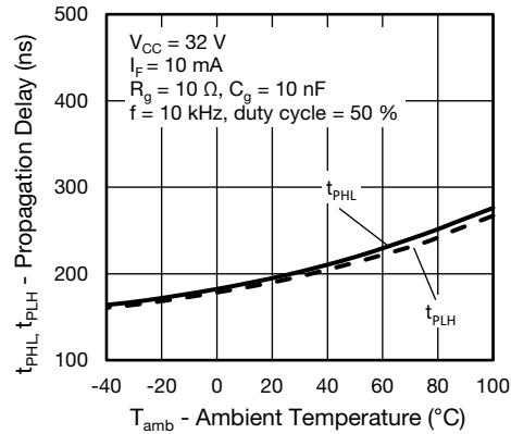
Fig. 18 - Propagation Delay vs. Ambient Temperature
