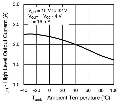
Fig. 8 - High Level Output Current vs. Ambient Temperature
