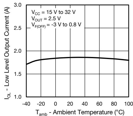
Fig. 10 - Low Level Output Current vs. Ambient Temperature
