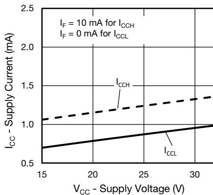
Fig. 14 - Supply Current vs. Supply Voltage
