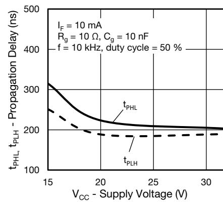
Fig. 17 - Propagation Delay vs. Supply Voltage
