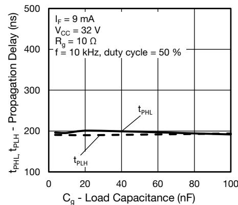
Fig. 21 - Propagation Delay vs. Load Capacitance
