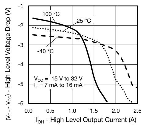
Fig. 12 - High Level Voltage Drop vs. High Level Output Current
