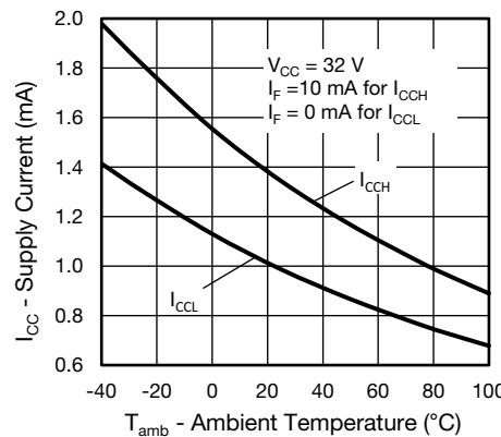
Fig. 13 - Supply Current vs. Ambient Temperature
