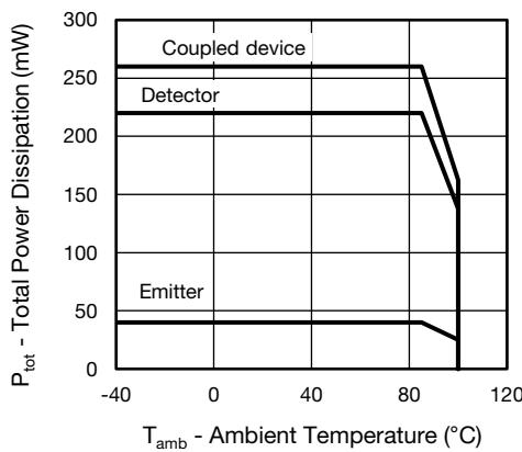
Fig. 3 - Power Dissipation vs. Ambient Temperature
