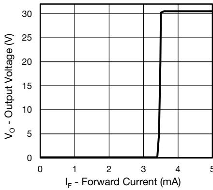
Fig. 16 - Output Voltage vs. Forward Current
