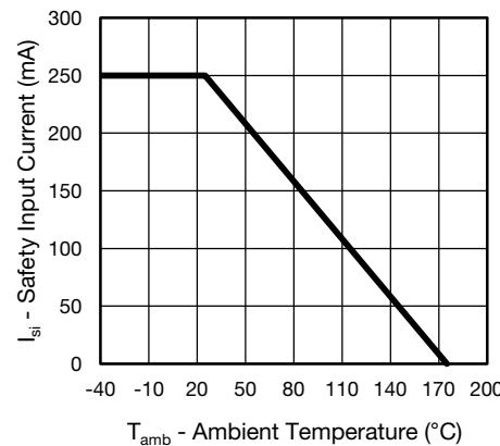
Fig. 2 - Safety Input Current vs. Ambient Temperature
