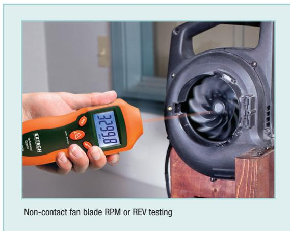
Non-contact fan blade RPM or REV testing
