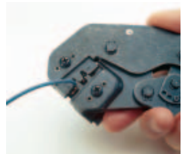
6. While pressing upward on the locator spring withdraw the crimp termination.
