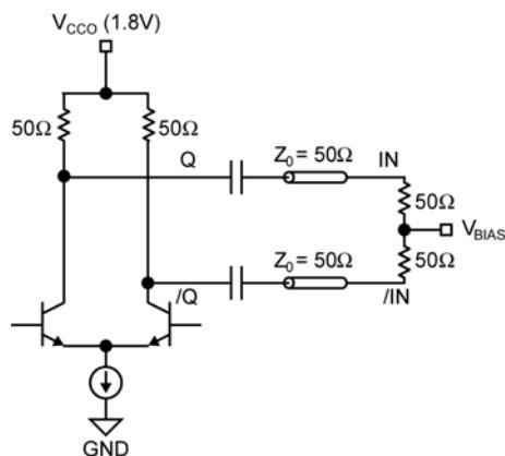
Figure 5c. CML AC-Coupled Termination
