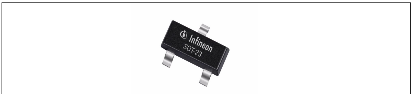
Figure 1-1 Image of TLE4964-1M in the PG-SOT23-3-15 Package
