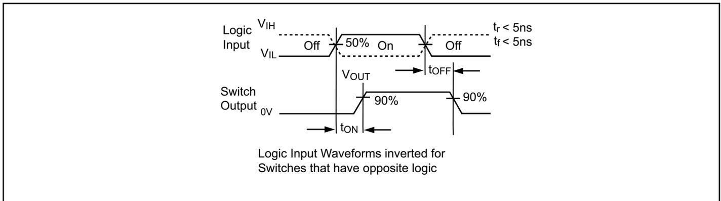
**Figure 2. AC Waveforms**
