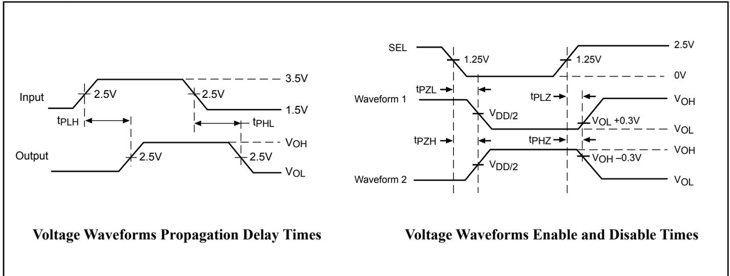
**Test Circuits and Timing Diagrams**
