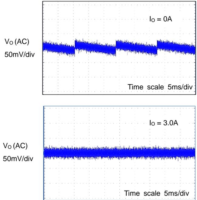
Figure 18. Output Voltage Ripple Wave
