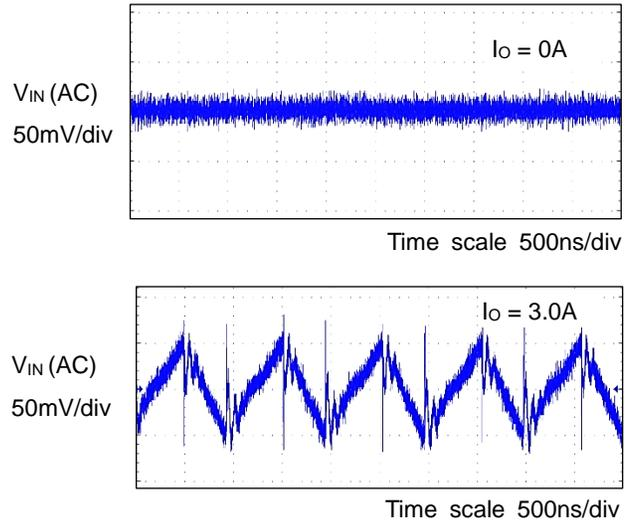
Figure 16. Input Voltage Ripple Wave
