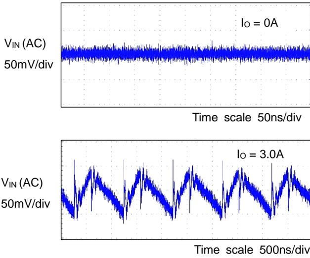
Figure 15. Input Voltage Ripple Wave
