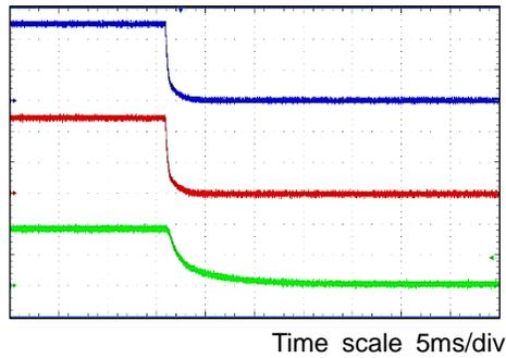
Figure 22. Power-down EN =  $V_{IN}$
