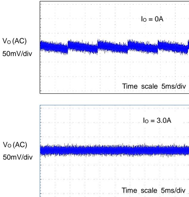
Figure 17. Output Voltage Ripple Wave
