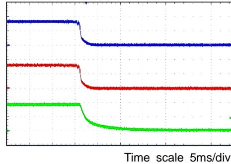
Figure 20. Power-down EN =  $V_{IN}$
