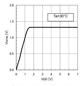
Fig2. Vtemp Voltage vs. Supply Voltage
