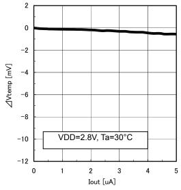
Fig4. Vtemp Voltage vs. Output Current
