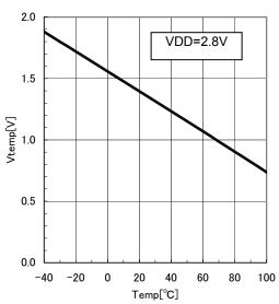
Fig3. Vtemp Voltage vs. Temperature
