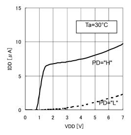
Fig1. Supply Current(IDD) vs. Supply Voltage
