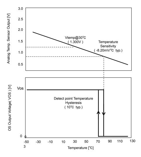
If the temperature over detect temperature, internal comparator operate OS output "H" to "L".(ex.active "L" Type) In case of OS return to "H",the temperature 10°C lower than detect temperature.
