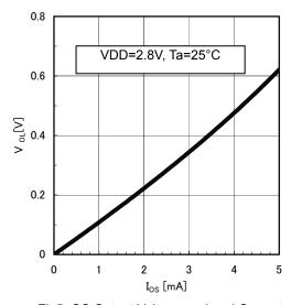
Fig5. OS Output Voltage vs. Load Current
