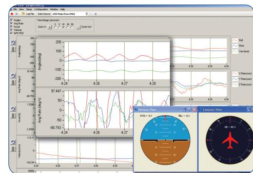
NAV-VIEW 2.0 provides an easy to use graphical interface to display, record and analyze all of the AHRS440 measurement parameters.
