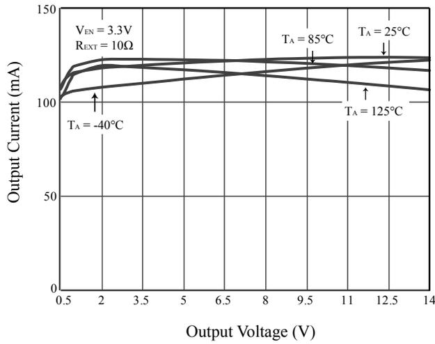
Figure 19  $I_{OUT}$  vs.  $V_{OUT}$
