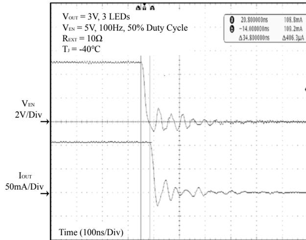
**Figure 35**  $V_{EN}$  vs.  $I_{OUT}$  Delay and Falling Edge
