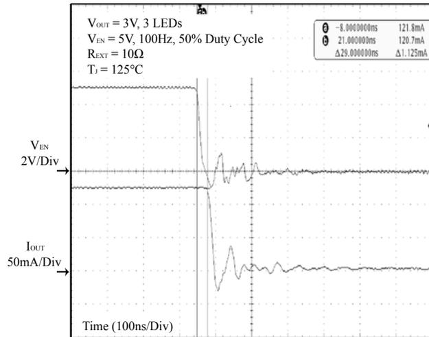
**Figure 37**  $V_{EN}$  vs.  $I_{OUT}$  Delay and Falling Edge
