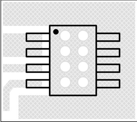
**Figure 40** Board Via Layout For Thermal Dissipation
