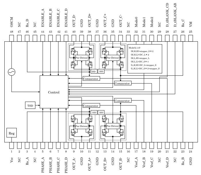
Note 1: GND wiring: We recommend that a heat sink be grounded at any parts, and the board and output pins be grounded at only one contact point. Take the heat dissipation into consideration when designing the board. When in controlling the setting pins for each mode by SW, those pins should be pulled up to power supply like V<sub>CC</sub> or pulled down to GND not to go into a high-impedance (Hi-Z) state.
