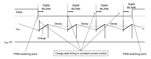
The digital tBLANK time is inserted immediately after the switching timing of externally applied PWM signals, IN1, IN2 and SB (such as the switching timing between short brake and charging), and also when the charging in constant-current chopper drive is started.
