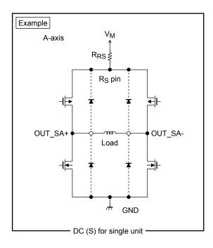
$\circ$   $\phantom{a}$  : Indicates an IC output pin connected to a motor.
