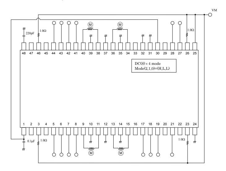
Note: Adding bypass capacitor is recommended if necessary. Make sure that GND wiring has only one contact point. To input the data, see the section on the recommended input data. If the signal setting is inappropriate, an unexpected large current may flow, causing damage to the IC.
