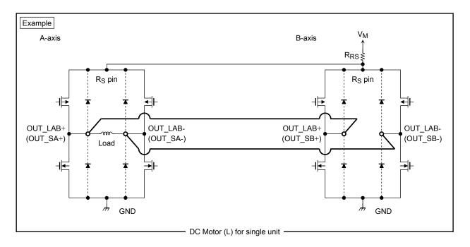
$\circ~$  : Indicates an IC output pin connected to a motor.
