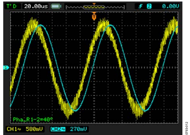
Figure 12. Phase Shift Between the AD2S1210 EXC and SIN Pins
