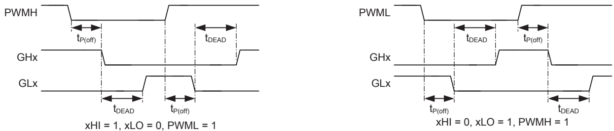
(B) Gate Drive Timing, PWM Inputs
