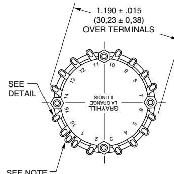
Note: Common location for a single pole per deck switch. For common location on multipole switches see circuit diagrams.
