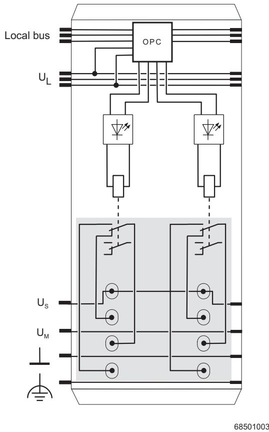
Figure 4 Internal wiring of the terminal points
