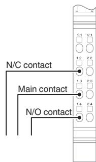
Figure 7 Actuator connection; floating connection
