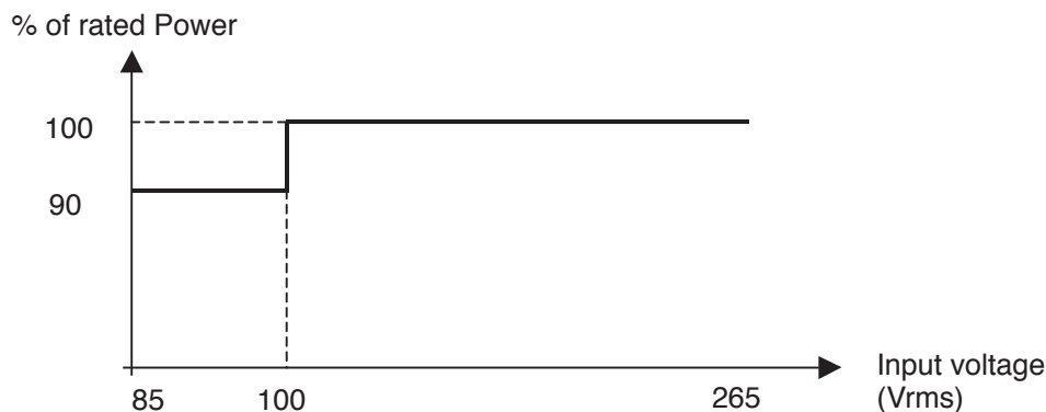
Fig 13-1: Output Power derating at parallel operation
