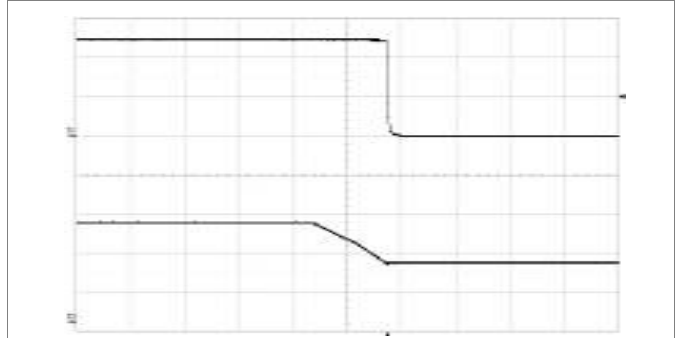
Shut-down enabled by disconnecting V_1 at: T_{P1} = +25^\circ\text{C} , V_1 = 53\text{ V} , I_O = 25\text{ A} resistive load. Top trace: output voltage (1 V/div.). Bottom trace: input voltage (20 V/div.). Time scale: (1 ms/div.).
