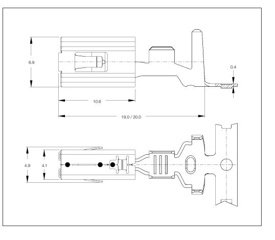
Mating Force: max. 16 N Unmating Force: max. 11 N Extraction Tool: Part No. 1-1579007-3 Product Group Drawing: 1241438
