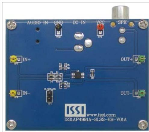
Figure 1: Photo of IS31AP4991A Evaluation Board (MSOP-8)
