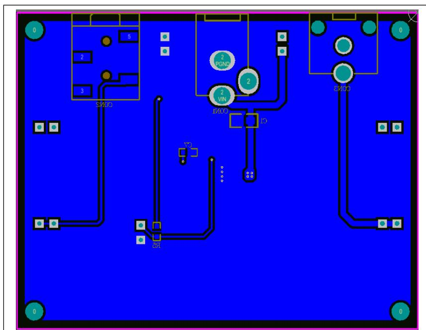
Figure 7: Board PCB Layout - Bottom Layer
