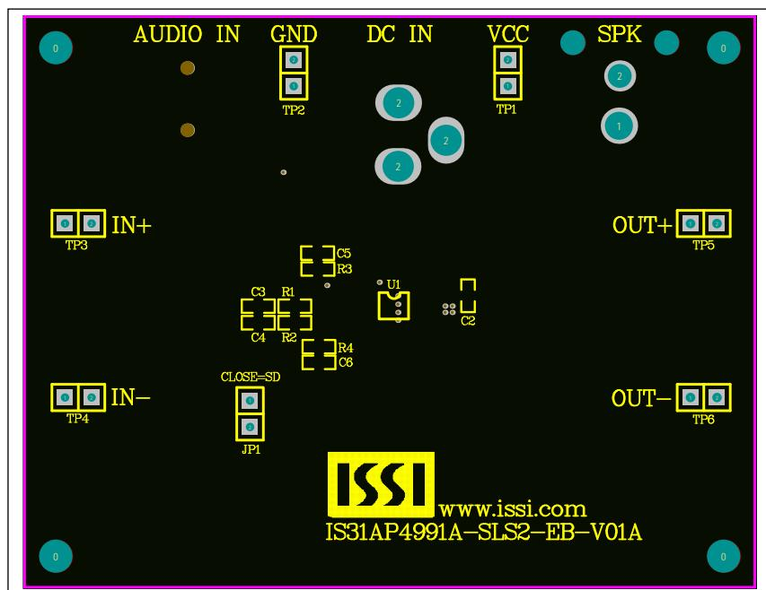
Figure 4: Board Component Placement Guide - Top Layer
