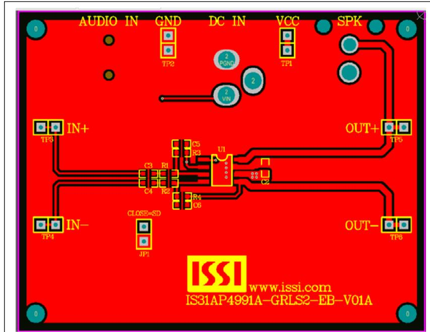
Figure 9: Board PCB Layout - Top Layer
