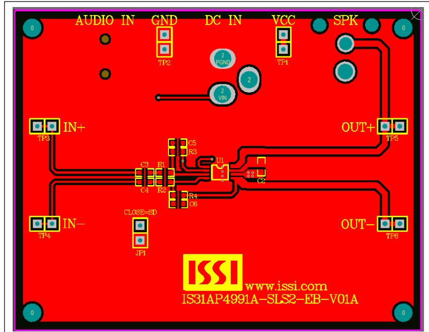
Figure 5: Board PCB Layout - Top Layer
