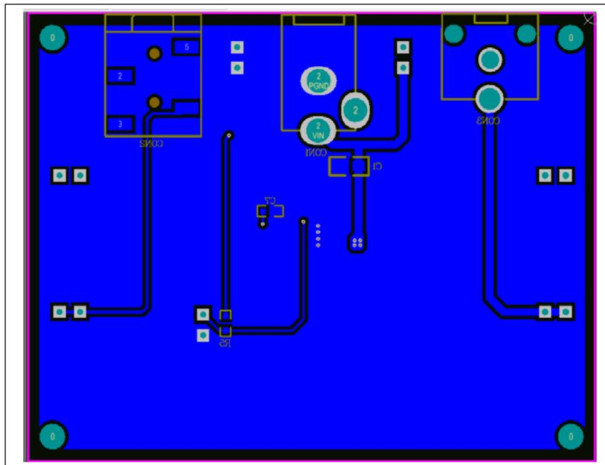
Figure 11: Board PCB Layout - Bottom Layer
