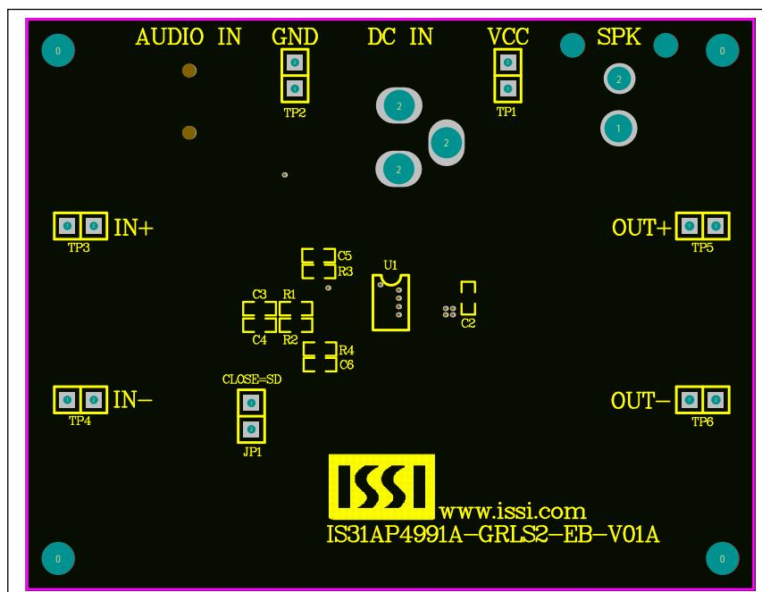
Figure 8: Board Component Placement Guide - Top Layer
