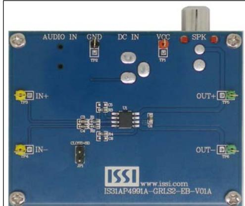
Figure 2: Photo of IS31AP4991A Evaluation Board (SOP-8)
