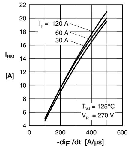
Fig. 3 Typ. reverse recov. current  $I_{RM}$  versus  $-di_F/dt$
