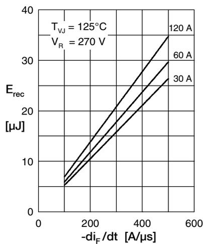
Fig. 7 Typ. recovery energy  $E_{rec}$  versus  $-di_F/dt$
