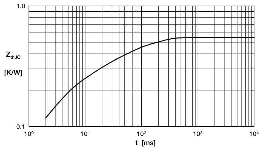
Fig. 8 Transient thermal impedance junction to case
