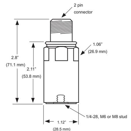
Accessories supplied: SF6 mounting stud; calibration data (level 2)
