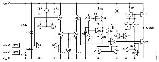
Figure 2. ADA4096-2 Simplfied Schemactic
