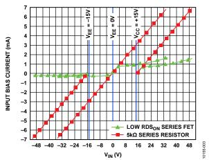
Figure 3. Input Current Limiting Capability
