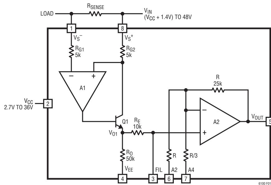
Figure 1. Functional Diagram
