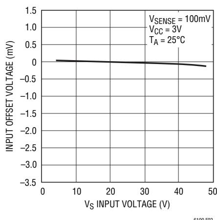
Figure 2.  $V_{\text{OS}}$  vs  $V_S$  Input Voltage
