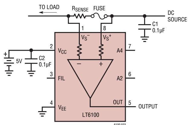
Figure 3. Current Monitoring of a Fuse Protected Circuit
