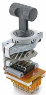
Lever switch, 2-5 positions, plug-in terminal, aluminium bezel, silver contacts, 33.5mm mounting
