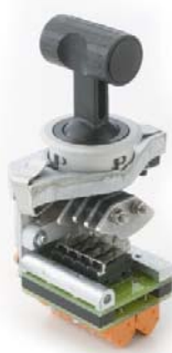
Lever switch, 2-5 positions, cage clamp®, aluminium bezel, silver contacts with positive opening, 33.5mm mounting
