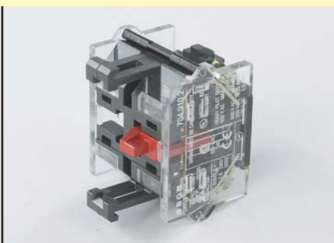
Contact block, screw terminal, slow-make with forced opening silver contacts
