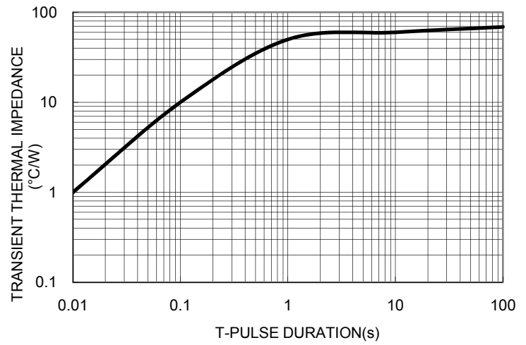
FIG. 6 TYPICAL TRANSIENT THERMAL IMPEDANCE PER LEG
