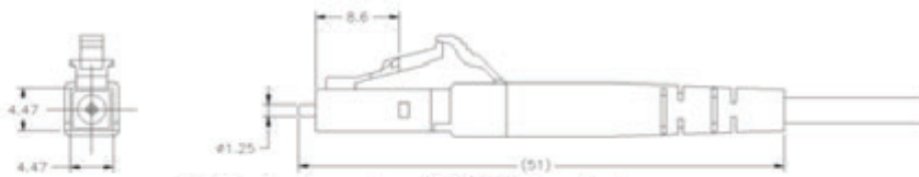
LC Simplex Connector with 1.6/2.0mm Boot
