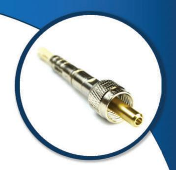
The connector ferrules is made from Beryllium Copper allowing the ferrule to act as a heat sink, pulling the heat quickly away from the fiber, when used. Damage threshold on these types of connectors will vary based on launch conditions and operational wavelength. The front body of the connector is a Beryllium Copper ferrule that is designed with a custom, high-tolerance, application-specific hole diameter.
