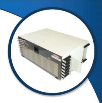
Panels are available with document cards for readily accessible port information. The 4RU Fiber Rack Mount Distribution Panels can accommodate from 6 to 288 fibers with optional LGX or high density adapter plates or cassettes with LC, MPO, SC, FC or ST adapters.
