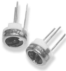
For applications that demand a durable, miniature trimming potentiometer, this military style offers quality at the right price. Cermet element technology ensures stability and performance in these 6mm diameter components. All units are fully sealed to withstand immersion in normal board washing solvents.
