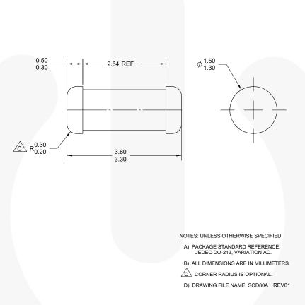
Figure 1. 2-TERMINAL, SOD-80, JEDEC DO-213AC, MINI-MELF
