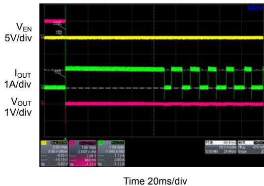
Figure 28. Output Short to GND Current ( V_{IN}=5V , C_{IN}=1.0\mu F )
