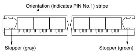
2) Tape and reel packing (surface-mount terminal type)
