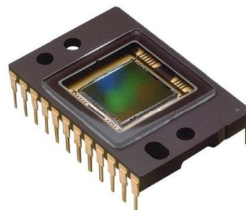
Figure 1. KAI-1010 Interline CCD Image Sensor
