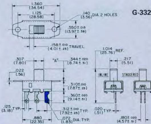
All switch types shown are illustrated in drawing. Single pole single throw versions have one end terminal (shown in blue) removed.
