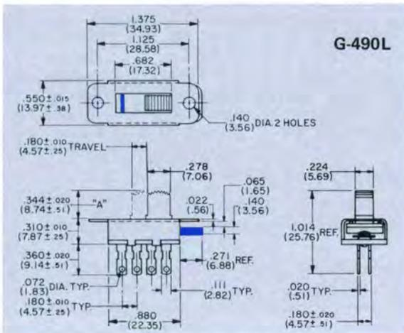
Switch shown in drawing is Type G-490L with button in extreme right position. The integral button cover closes the entire opening at the top of the switch and extends outside the end of the housing as shown in blue. If covering the opening at the top of switch is not necessary, specify G-490S. Drawing of G-490S has blue line in top view showing that extension outside the end of the switch housing is omitted.
