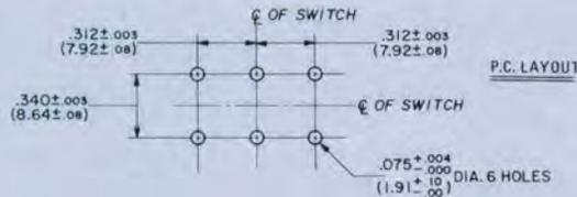
**TWIST TAB** • Mount to .031" thick metal chassis by specifying housing G-01-112. Housing ears, when twisted in chassis cutout shown, lock switch into place. See drawing on page 11.
