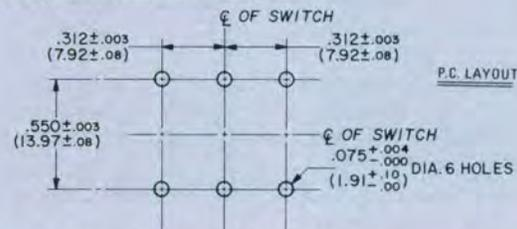
**TWIST TAB** • Mount to .031"-.047" thick metal chassis by specifying bracket G-10-11. Housing ears, when twisted in chassis cutout shown, lock switch into place. See drawing on page 16.
