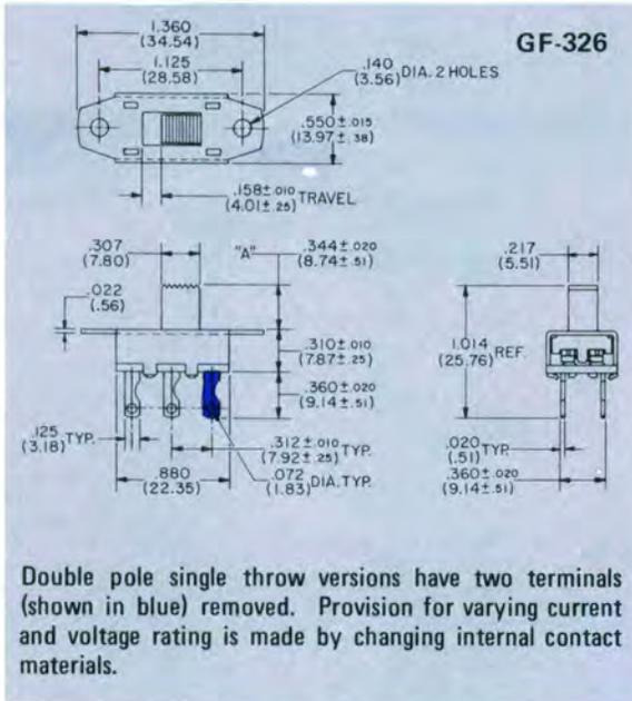
Double pole single throw versions have two terminals (shown in blue) removed. Provision for varying current and voltage rating is made by changing internal contact materials.
