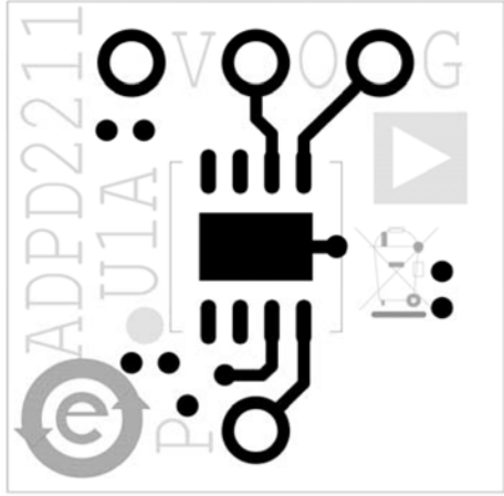
Figure 15. ADPD2211 Evaluation Board Top Layer
