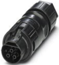
PRC connector, black, 3-pos., 1.5 mm<sup>2</sup> ... 6 mm<sup>2</sup>/630 V/35 A, with screw connection, for cables with a diameter of 8 mm ... 21 mm.
