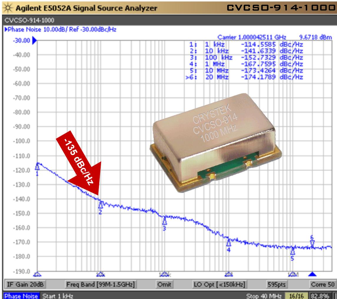
Model CVCSO-914-1000 is a 1 GHz voltage-controlled SAW (surface acoustic wave) Clock Oscillator (VCSO). SAW crystal technology provides low-noise and low-jitter performance with true sinewave output. Features include -135 dBc/Hz phase noise at 10 kHz offset, 5V input voltage, -20°C to +70°C operating temperature, and 9×14 mm SMT package. The oscillator has no sub-harmonic and the second harmonic is typically -20 dBc.
