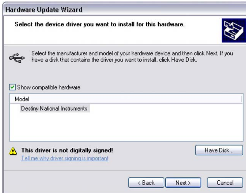
Figure 2-7. Selecting the “Destiny National Instruments” Driver
